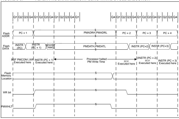
An example of the complete four-word write sequence is shown in Example 3-2. The initial address is loaded into the PMADRH and PMADRL register pair; the eight words of data are loaded using indirect addressing.
