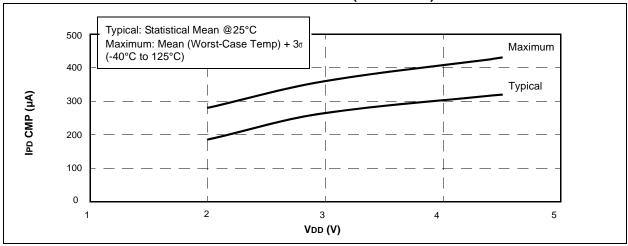
FIGURE 17-28: PIC12HV609/615 IPD WDT vs. VDD
