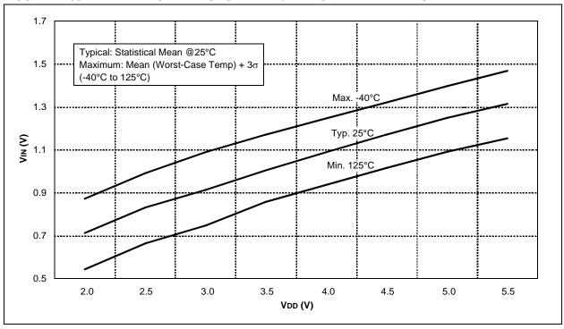
FIGURE 17-39: SCHMITT TRIGGER INPUT THRESHOLD VIN vs. VDD OVER TEMPERATURE 4.0 Typical: Statistical Mean @25°C 3.5 Maximum: Mean (Worst-Case Temp) + 3σ (-40°C to 125°C) 3.0 2.5 Vin (V 2.0 VIL Max. -40°C 1.5 VIL Min. 125°C 1.0 0.5 2.0 2.5 3.0 3.5 4.0 5.0 5.5 4.5 VDD (V)
