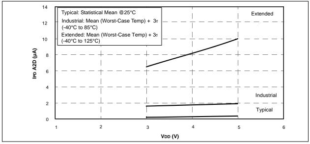
FIGURE 17-18: PIC12HV609/615 IDD LP (32 kHz) vs. VDD
