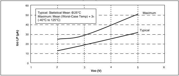
FIGURE 17-2: PIC12F609/615/617 IDD EC (1 MHz) vs. VDD
