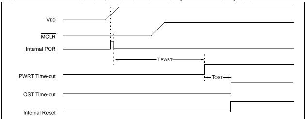
FIGURE 12-5: TIME-OUT SEQUENCE ON POWER-UP (DELAYED MCLR): CASE 2
