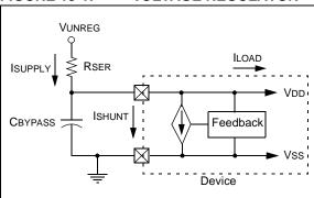
An external current limiting resistor, RSER, located between the unregulated supply, VUNREG, and the VDD pin, drops the difference in voltage between VUNREG and VDD. RSER must be between RMAX and RMIN as defined by Equation 13-1.
