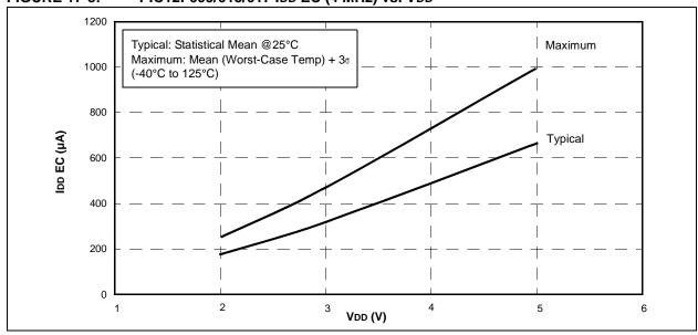
FIGURE 17-4: PIC12F609/615/617 IDD XT (1 MHz) vs. VDD
