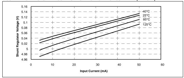
FIGURE 17-50: SHUNT REGULATOR VOLTAGE vs. TEMP (TYPICAL)
