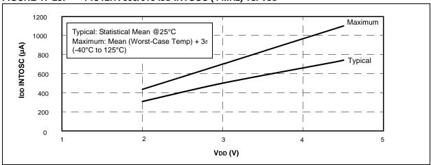
FIGURE 17-24: PIC12HV609/615 IDD INTOSC (8 MHz) vs. VDD
