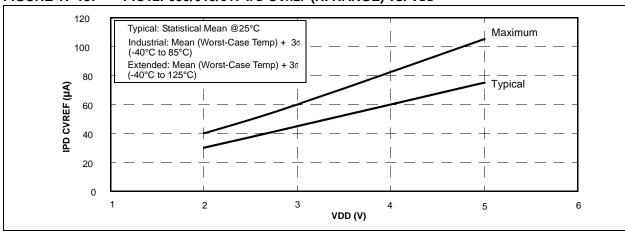
FIGURE 17-16: PIC12F609/615/617 IPD T1OSC vs. VDD
