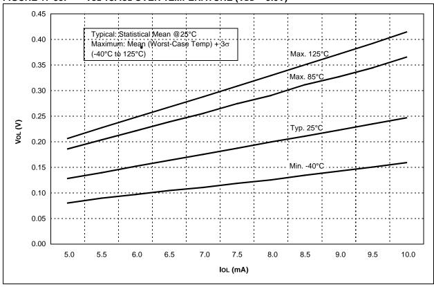
FIGURE 17-36: Voh vs. Ioh OVER TEMPERATURE (VDD = 3.0V)
