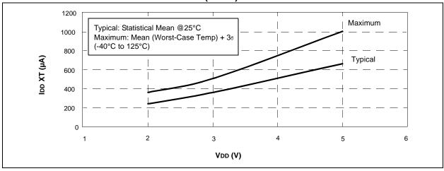
FIGURE 17-6: PIC12F609/615/617 IDD INTOSC (4 MHz) vs. VDD
