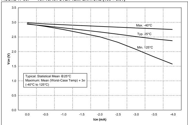
FIGURE 17-37: VOH vs. IOH OVER TEMPERATURE (VDD = 5.0V)
