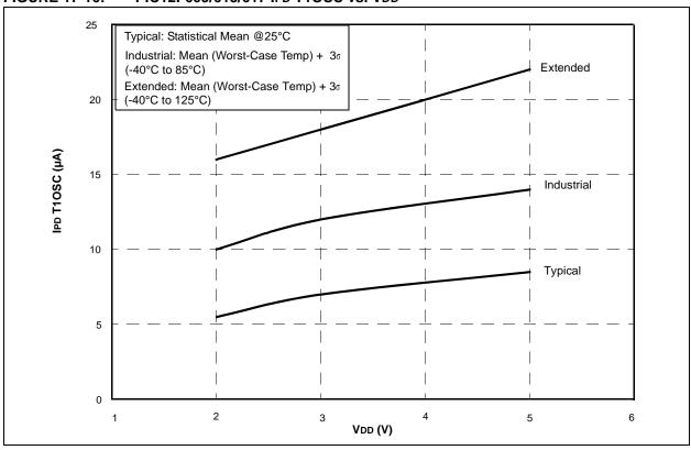
FIGURE 17-17: PIC12F615/617 IPD A/D vs. VDD
