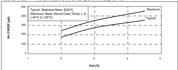
FIGURE 17-31: PIC12HV609/615 IPD CVREF (HI RANGE) vs. VDD
