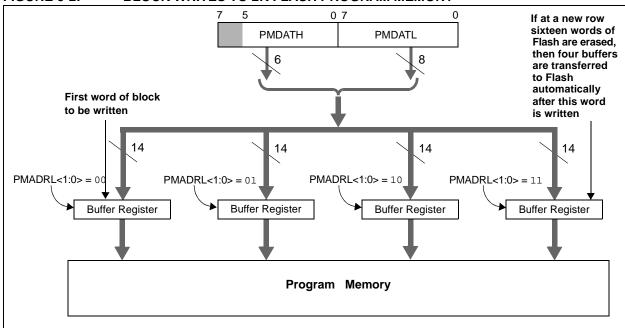
FIGURE 3-3: FLASH PROGRAM MEMORY LONG WRITE CYCLE EXECUTION
