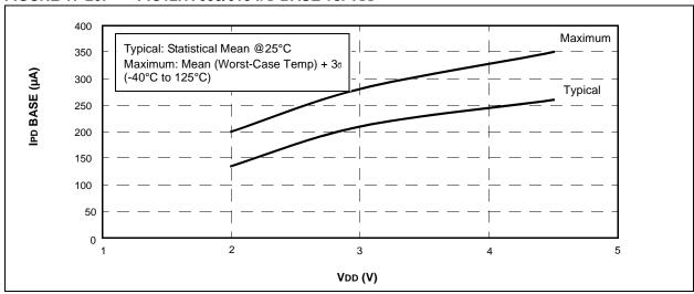
FIGURE 17-27: PIC12HV609/615 IPD COMPARATOR (SINGLE ON) vs. VDD
