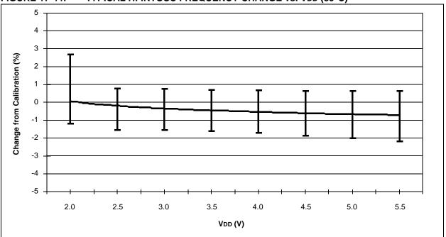
FIGURE 17-45: TYPICAL HFINTOSC FREQUENCY CHANGE vs. VDD (125°C)
