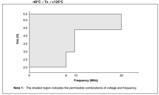
FIGURE 16-2: PIC12HV609/615 VOLTAGE-FREQUENCY GRAPH,  $-40^{\circ}\text{C} \le \text{Ta} \le +125^{\circ}\text{C}$
