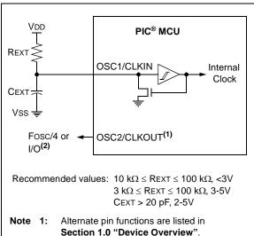
In RCIO mode, the RC circuit is connected to OSC1. OSC2 becomes an additional general purpose I/O pin.
