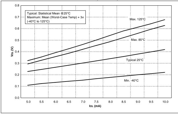
FIGURE 17-35: Vol vs. Iol OVER TEMPERATURE (VDD = 5.0V)
