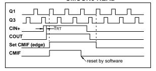
FIGURE 9-5: COMPARATOR INTERRUPT TIMING WITH CMCON0 READ
