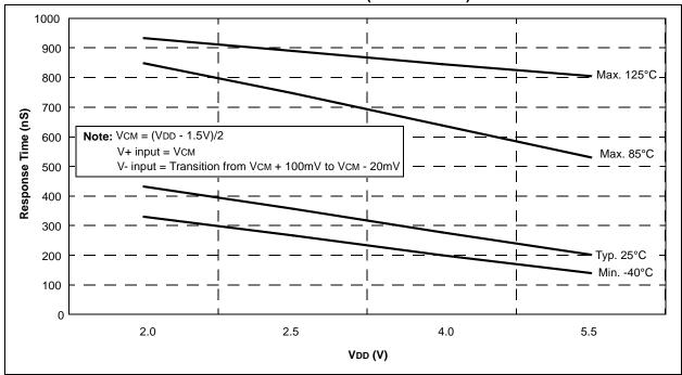
FIGURE 17-52: **COMPARATOR RESPONSE TIME (FALLING EDGE)** 1000 900 Max. 125°C-800 700 Response Time (nS) 600 **Note:** VCM = (VDD - 1.5V)/2V+ input = VCM 500 V- input = Transition from VcM - 100mV to VcM + 20MV 400 300 Typ. 25°C 200 Min. -40°C 100 0 2.0 2.5 4.0 5.5 VDD (V)
