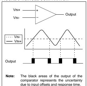
FIGURE 9-2: COMPARATOR SIMPLIFIED BLOCK DIAGRAM
