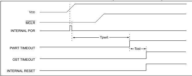
FIGURE 14-9: TIMEOUT SEQUENCE ON POWER-UP (MCLR NOT TIED TO VDD): CASE 2
