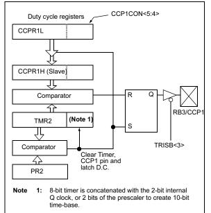
A PWM output (Figure 11-3) has a time-base (period) and a time that the output stays high (duty cycle). The frequency of the PWM is the inverse of the period (1/period).
