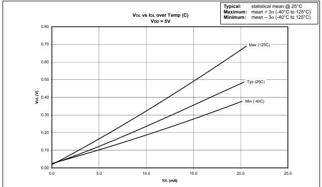
FIGURE 18-20: VOL VS IOL OVER TEMP (C) VDD = 5V
